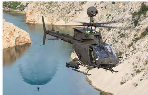
Above: The mast-mounted sight enables the Kiowa Warrior crew to remain hidden and peek at targets without revealing themselves.
