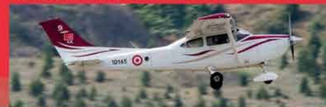
Above: The latest addition to the fixed-wing fleet of the Army Aviation School is the Cessna T182T Skylane. Featuring a digital cockpit and the Garmin 1000 system, it is well equipped for training pilots. Below: From 1991 onwards, the Turkish Armed Forces received seven Beech B200 twin-engine aircraft. Two are operated by Milli Savunma Bakanlığı (Ministry of Defence), four are operated by the Army while one crashed in 1992.
