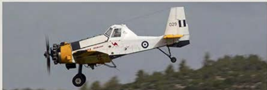
Above: Serial 029 (c/n 12010-29), a single-seat M-18B, approaches a practice target at very low level. Dromader pilots work at extremely low level, making them just as effective as a CL-415 dropping four times the amount of water from a slightly higher altitude. Below: Squadron commander Vasileios Theodorakis in front of his aircraft.
